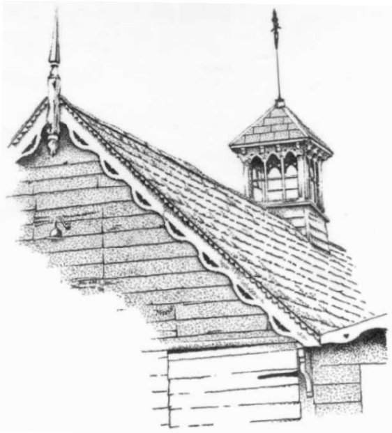
Decorative finial and bargeboard detail at Ivy House Workshop, Bridge Road.
